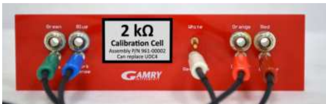
Figure 4-2 2 k \Omega Calibration Cell with Leads Attached for Calibration
