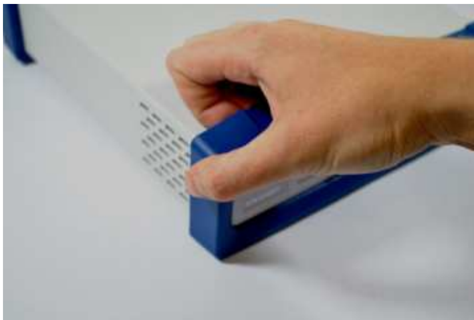
Figure 3-5 Removing the Front Bezel
