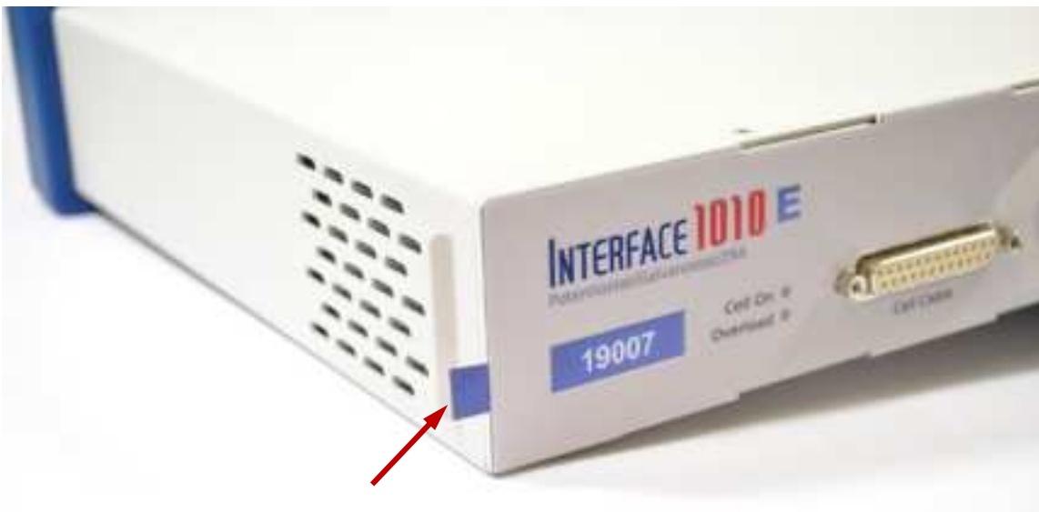
Figure 3-6 Instrument with Bezel Removed - Label Tab is Visible
