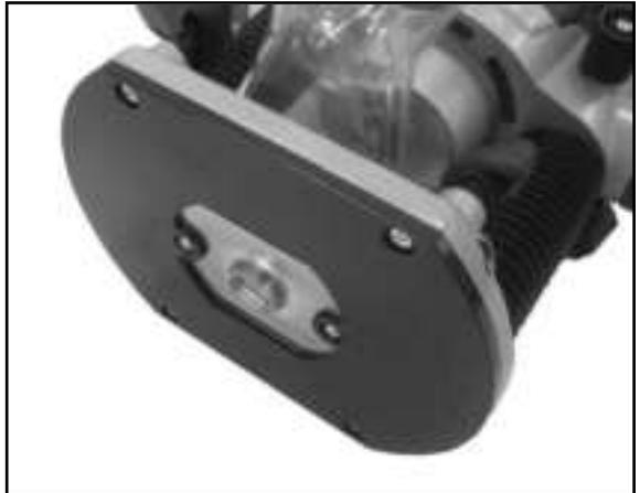
Switch on the router. Loosen retaining lever (14) and slowly lower the router to the workpiece until the adjusted depth-of-cut is reached. Re-tighten the retaining lever (14).
