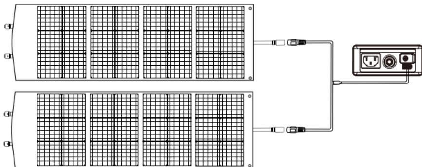
2. If using MC4 cables for parallel connection:
