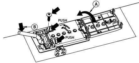
**The appliance must be connected to the electricity supply by means of an all-pole disconnect switch with minimum contact gap of 3 mm.**
