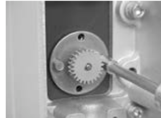
Remove Packing Gland Mounting Screws
