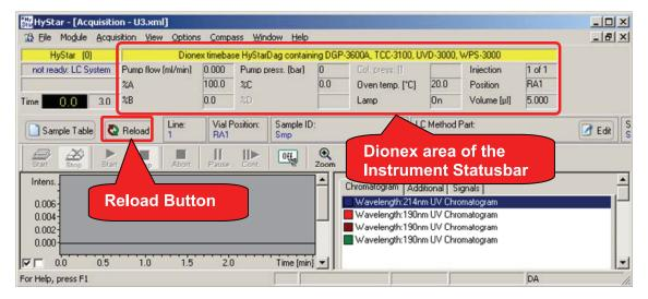
The Instrument Statusbar in the HyStar Acquisition module shows information about the instruments attached to the system. The Dionex area shows the status of DCMS<sup>Link</sup> as follows:
