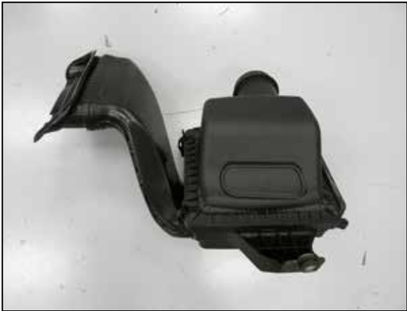
7. Remove the air filter housing/fresh air intake duct assembly from the vehicle.
