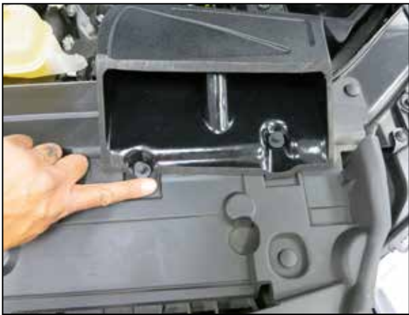
14. Secure the fresh air intake duct with the provided push pins.
