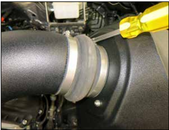
21. Install the K&N intake tube onto the throttle body and filter adapter, adjust for best fit and then secure with the provided hose clamps.
