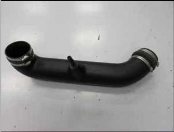
20. Install the couplers onto the K&N intake tube and secure with the provided hose clamps.
