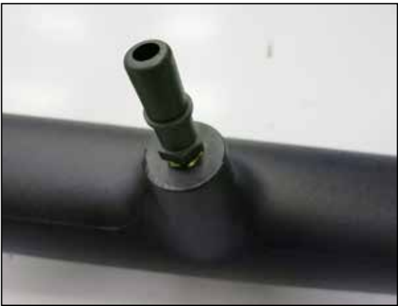
19. Install the provided CCV quick connect fitting into the K&N intake tube.
