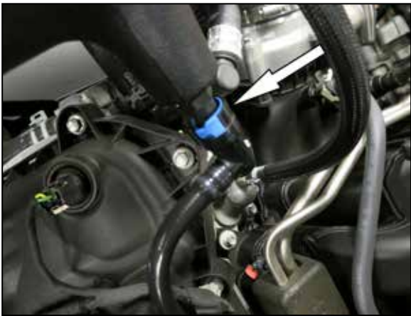
22. Connect the factory CCV hose to the quick connect fitting installed into the K&N intake tube.
