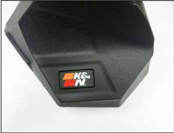
15. Snap the K&N badge into the upper air filter housing.
