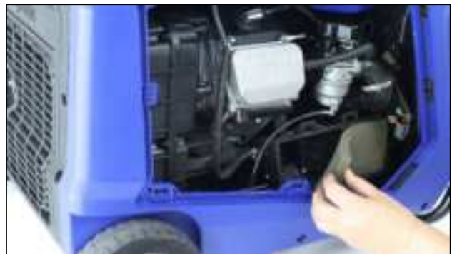
Figure 37 Remove the Air Filter Element
