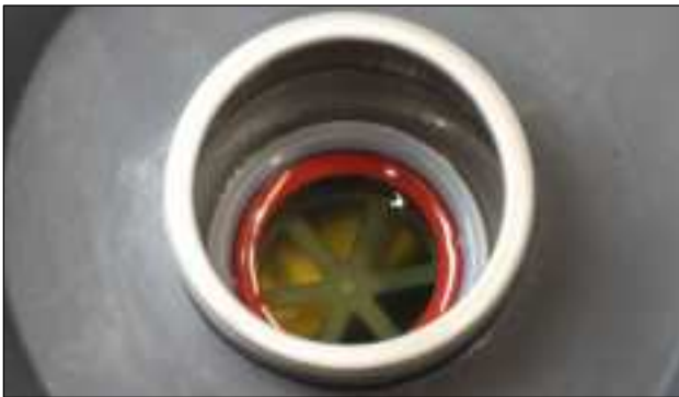
Figure 12 Maximum Fuel Fill Level
