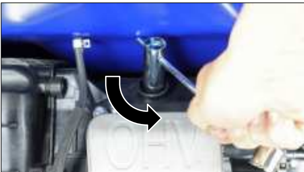
Figure 44 Remove the Spark Plug
