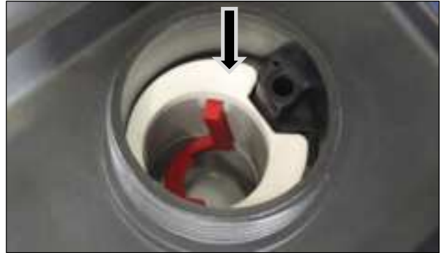
Figure 39 Install the Fuel Strainer
