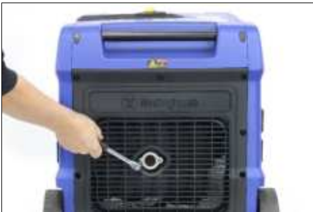
Figure 46 Remove the Spark Arrestor Clamp
