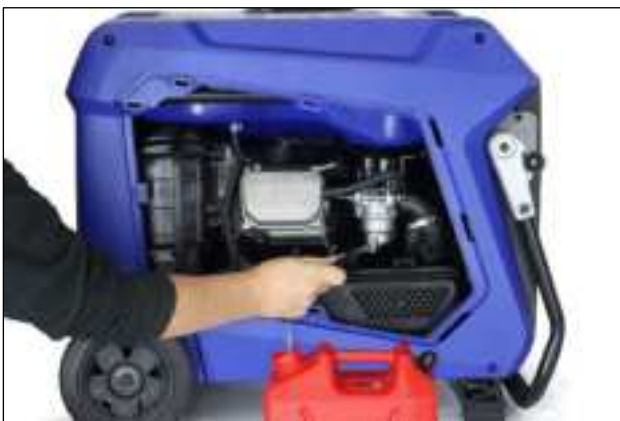
Figure 41 Drain the Carburettor
