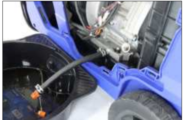
Figure 33 Draining the Engine Oil
