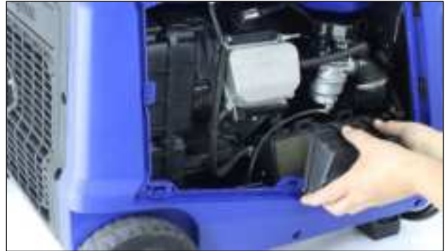
Figure 36 Remove the Air Filter Cover
