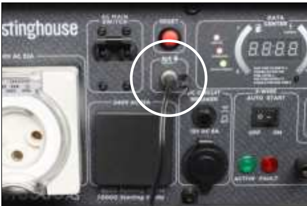
Figure 34 Connecting the Battery Charger to the Generator
