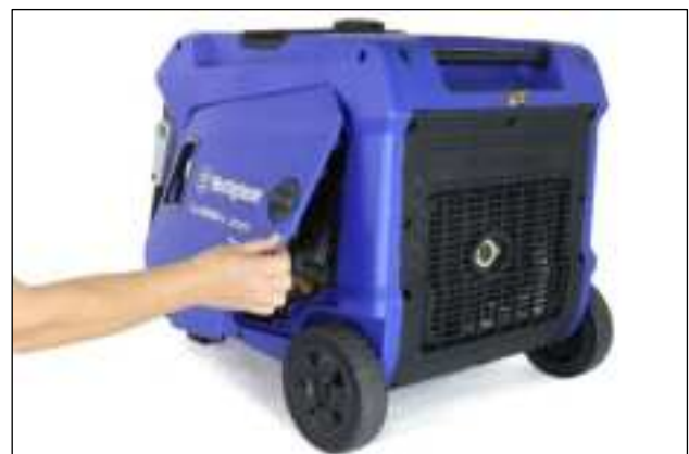
Figure 27 Remove the RHS Access Cover
