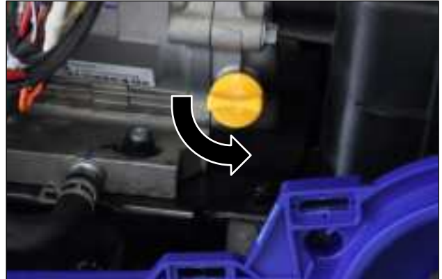
Figure 30 Remove the Oil Fill Plug
