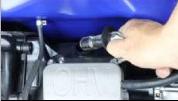
Figure 43 Remove the Spark Plug Boot
