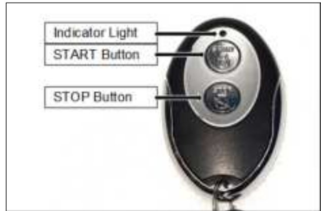
Figure 18 Wireless Remote Control Fob
