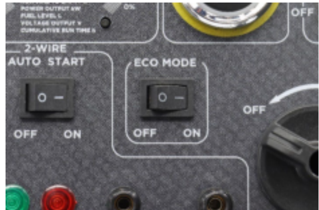
Figure 20 ECO Mode Switch in the ON Position
