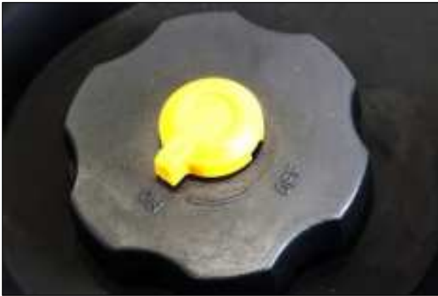
Figure 11 Fuel Cap Vent in the ON Position
