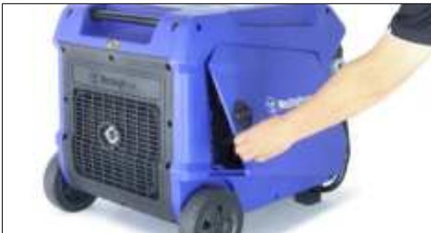
Figure 29 Remove the LHS Access Cover
