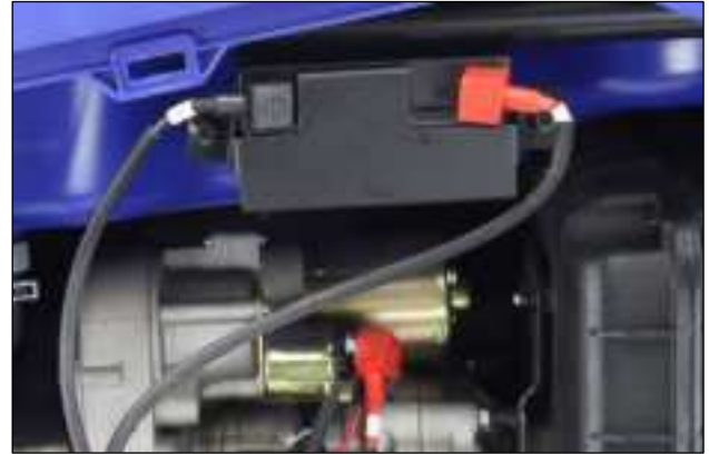
Figure 7 Battery Mounting Inside Generator
