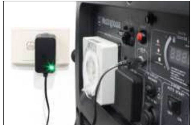
Figure 35 Connecting the Battery Charger to Mains Power Supply
