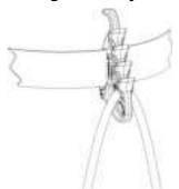
Start by pushing the trailing end of the lanyard rope, into the bottom slot of the NESSIE.
