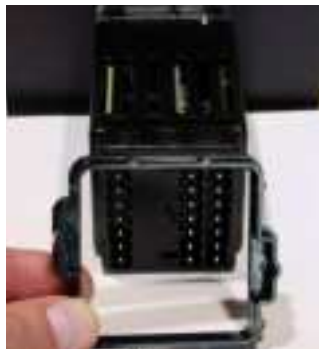
Figure 2: Slide Mounting Bracket over Controller
