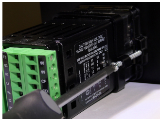
Figure 3: Tighten the Mounting Screws
