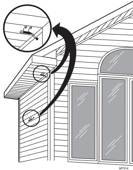
Fig. 27. Typical locations for C7089U1006 Outdoor Sensor.
