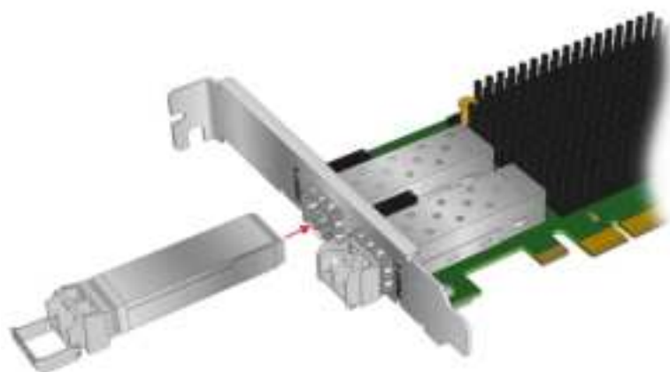
Figure 5: Installing an Optical Transceiver
