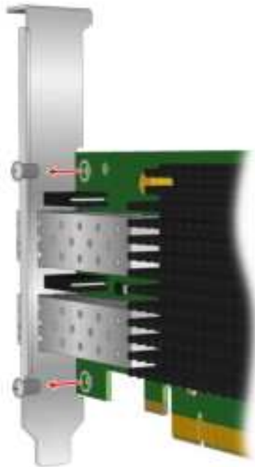
Figure 4: Removing the Mounting Bracket
