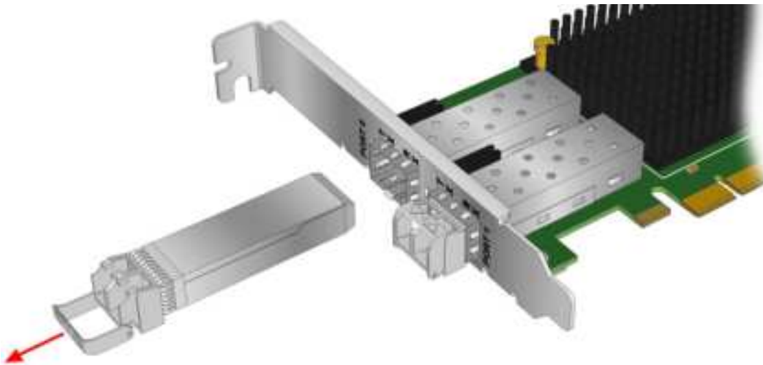
Figure 3: Removing an Optical Transceiver
