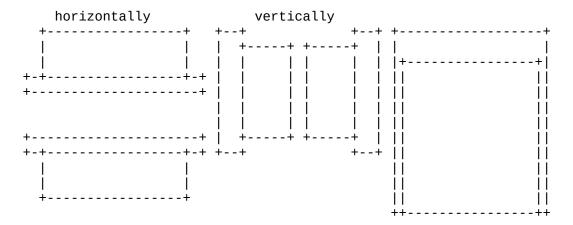
You can mount the disk drive in any position. R models mount in RAID storage subsystems. The drive (with bezel) attaches to the system bay and accept #6-32 screws. Screws should not exceed 0.25 inch (6.25 millimeters) in length, otherwise damage to the PCB may result.
