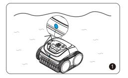
About 20 seconds of auto calibration on the floor, the indicator light will turn flashing blue. The cleaner is ready to clean.
