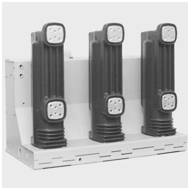
Figure 9/4: Vacuum circuit-breaker, type VM1, high-current, for fixed installation, 12 kV, 1600...2000 A, \leq 40 kA, pole side.
