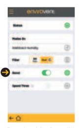
To put the unit into Boost, slide the Boost toggle to the ON position. The Boost run on time is set on the Setting Page. Boost can be turned off at any time. Please note that boost cannot be activated whilst the unit is in Speed Three.
