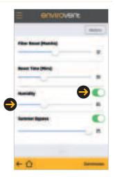
Humidity can be set to 55, 65, 75 and 85%. Factory default is 65%. In installer mode only, humidity can be deactivated. Press **Save** to confirm changes.
