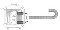
Choose a nozzle based on the items being inflated or deflated, horizontally align the hose and accessory nozzle, twist them clockwise along the threads.
