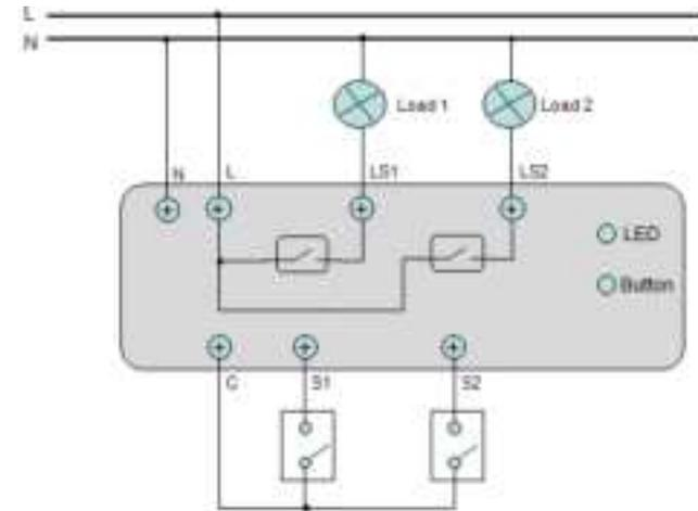
**Warning: The external switches cannot be connected to the load directly.**
