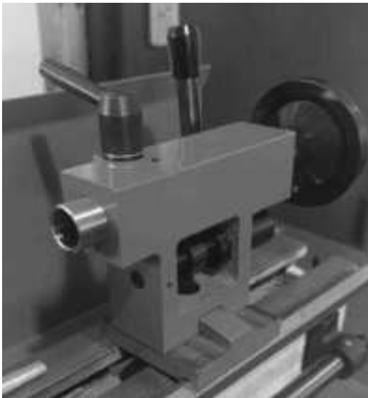
A Fig.3 Tailstock Rest Adjustment
