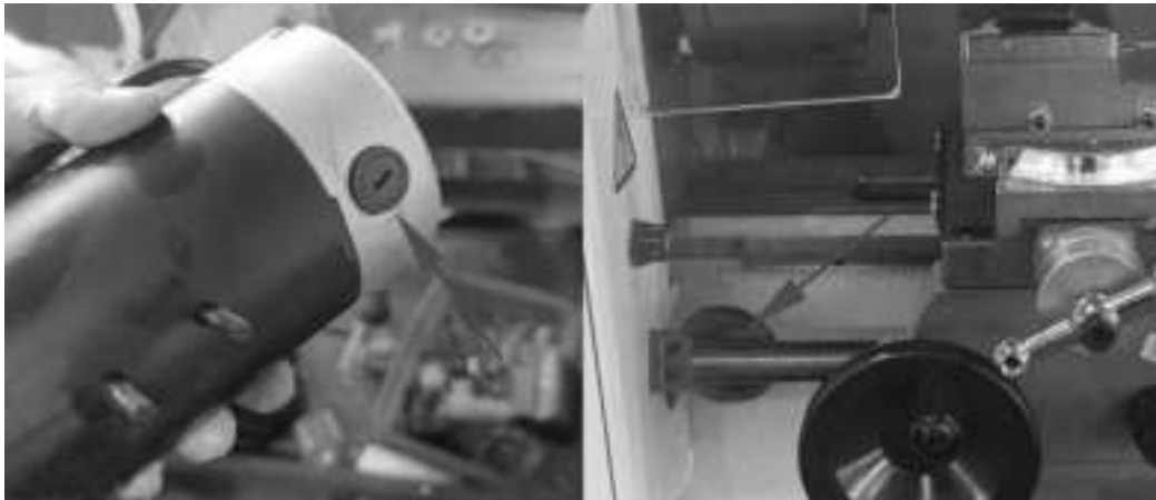
A Fig.4 Replacement of carbon brushes
