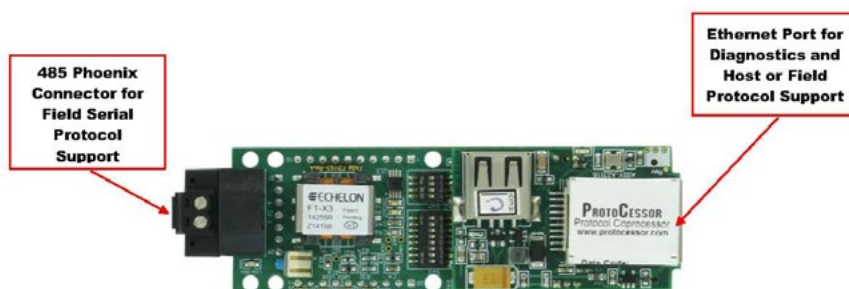
Figure 18: PT-Link II LON-3® Components
