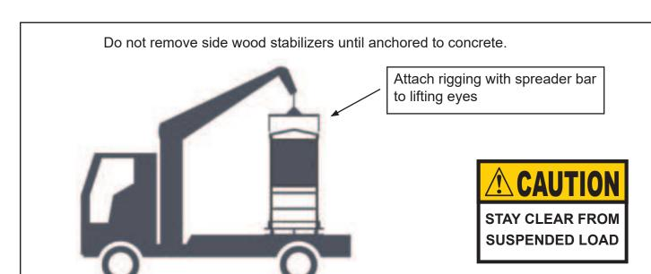
LIFTING EYE CAPACITY: 700lbs combined max
