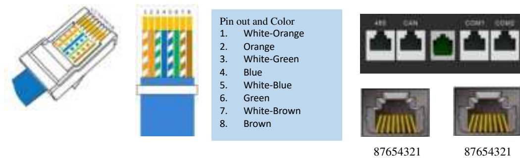
Figure 2-2 CAN,RS485,COM1,COM2 interface definition
