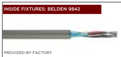
FIGURE A - USING SHIELDED TWISTED PAIR WIRE WILL REDUCE THE RISK OF EXTERNAL INTERFERENCE PICK-UP (I.E. FLICKERING, STROBING, ETC)
