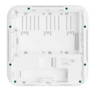
**7.** Slide the latches and carefully remove both boards, keeping them in the same plane and not disconnecting them. There are connectors between boards; do not break them.
