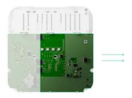
8. Disconnect the power supply unit (the larger board) from the main board.
