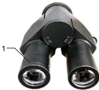
Fig. 10. Adjusting the diopter adjustment mechanism
