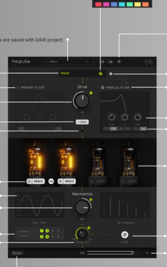
Track colour will be assigned from daw automatically if daw supports, otherwise use palette to manually select colour. Colour is used in hardware knob control assigns.
