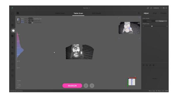
The ruler on the left side shows the scanning distance you keep. And the waveform represents whether the distance is appropriate or not.
