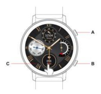
Button A: Long press to switch ON/OFF, short press to turn ON/OFF the screen.
