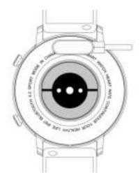
\* Please note that the two contacts of the charging cable cannot contact the conductor at the same time, which will cause the circuit to burn.
