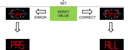
When in Pr2, the label of all parameters in Pr1 will have the "decimal point". The level Pr2 will be accessible until exiting programming mode.
