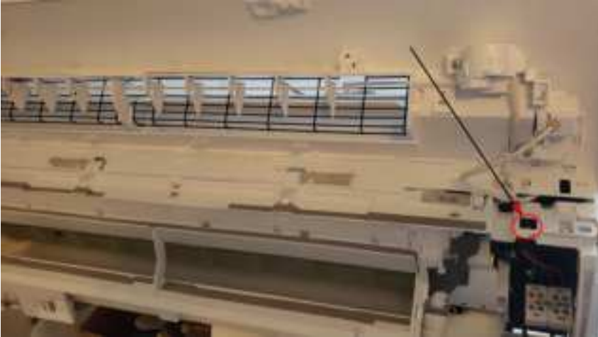
Fig. 510 (Door Micro Switch)
