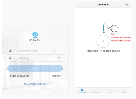
5. Click the monitoring interface and set the user and password as shown in the following figure (the default password is empty when the device is manufactured, which needs to be set before it can be used).
