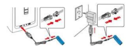
4. Once charging is complete, connect the battery to the correct electrodes in the battery compartment. Replace the battery cover and secure it with the previously removed screw.
