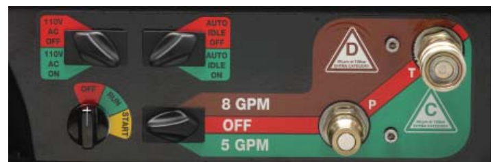
Figure 1. Panel Control Valve
