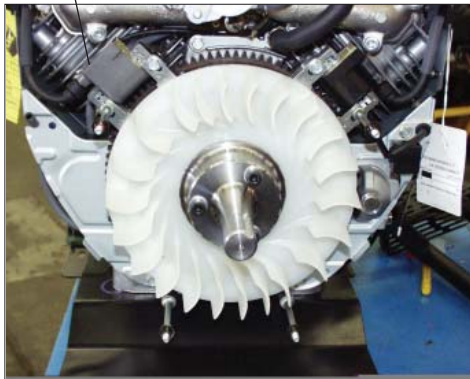
Location of Magnetgo Wire Connection
