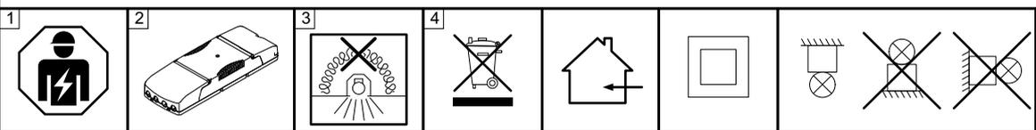
**EN** 1 **The installation and commissioning** of the luminaire as well as any modification to the luminaire may only be performed by authorized personnel (qualified electrician).
