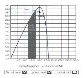
Figure 1-2 Maximum Power Point Curve
