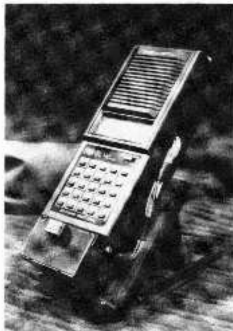
An external view of the PRO-34 set up for 3,200 channel operation. The external cable bundle (and the Memory Chip) can probably be wired and routed internally if you are willing to use external power and forget the battery pack.
