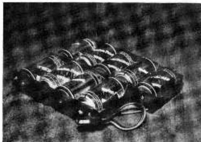
Homemade 13.5 VDC alkaline battery pack. Two four-cell packs are glued together and rewired to make a nine-cell (13.5 volt) pack.
