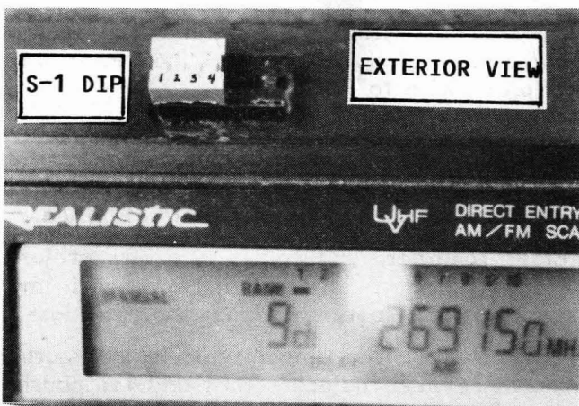
An external view of the 4-segment DIP switch, showing its installation. The author used a 16-pin socket for other purposes. You need only an 8-pin socket for this modification.
