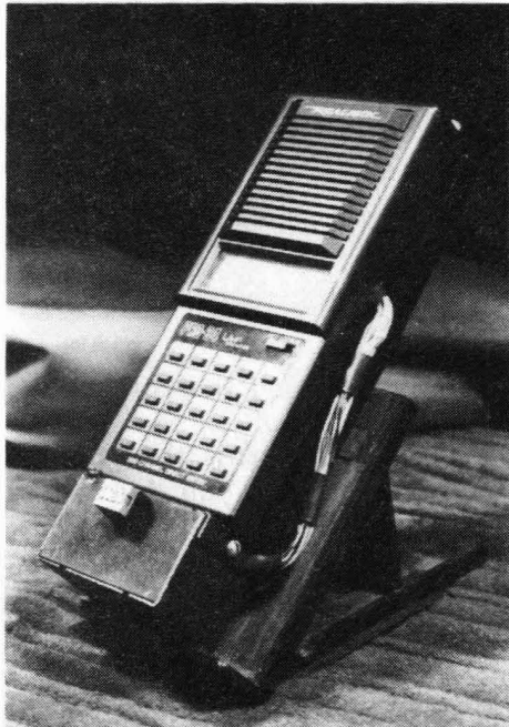
An external view of the PRO-34 set up for 3,200 channel operation. The external cable bundle (and the Memory Chop) can probably be wired and routed internally if you are willing to use external power and forget the battery pack.
