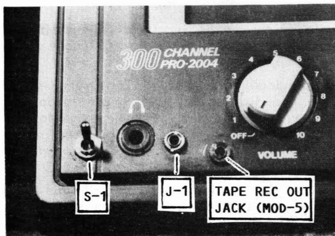
Front panel of the PRO-2004 showing the mounting of the new tape recorder switch (at left) and new TAPE REC out jack from MOD-5.
