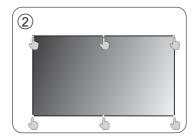
2. First of all, pull the screen fabric flat and lay it on the wall where it will be installed. Mark every position of the grommets correctly on the wall.
