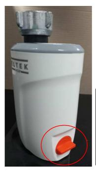
In case of flow anomaly turn the orange lever clockwise 90° and release it to reset the device.
