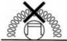
The power supply (LED Drive) that can be used where normally flammable materials including building insulation, are or may be present, but cannot be abutted against any material and cannot be covered in normal. Minimum clearance distance from the top and sides of the control gear to normally flammable building element is 75 mm; as shown in below picture,  $A=B=C=\text{Min. } 75 \text{ mm}$ .
