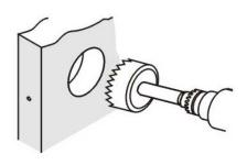
Drill 1" (25mm) hole in center of door edge through to 2-1/8" (54mm) hole for latch.
