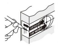
Mark center hole on door face through guide on template for either 2-3/8" (60mm) or 2-3/4" (70mm) backset.
