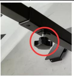
Step 4: Install the retractable brackets with M8 34mm plastic screws. The height of the retractable brackets can be adjusted at any length.
