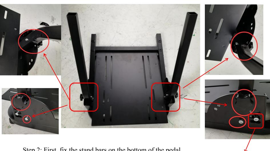
Step 2: First, fix the stand bars on the bottom of the pedal with two M8 60mm plastic screws. Then use two M8 56mm screws (for both sides) to lock the stand bars with nuts.
