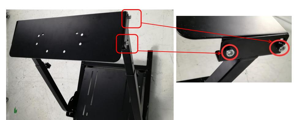
Step 5: Install the steering wheel base on the top of the retractable brackets with four M8 22mm screws (two screws for each side), and then fix it with nuts.
