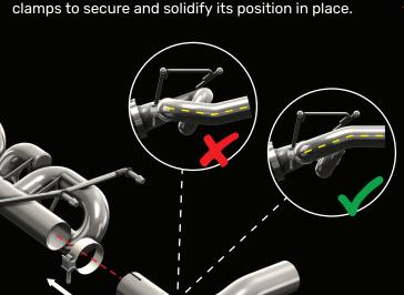
Lastly, the tips. Slide the tips over the tailpipes and center the "J" logo to the top so the angle of the tip is symmetrical. Adjust the depth of the tip to your liking and then tighten the slip joint clamp to secure its position. Take a step back and evaluate both tips to ensure they are symmetrical and leveled as you may need to loosen the clamps to make minor adjustments prior to tightening them again.
