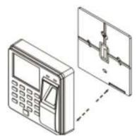
3. Align the holes drilled in the wall and screw the back cover to the wall with Screws
