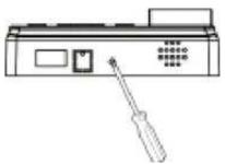
2. Remove the back cover from the device
