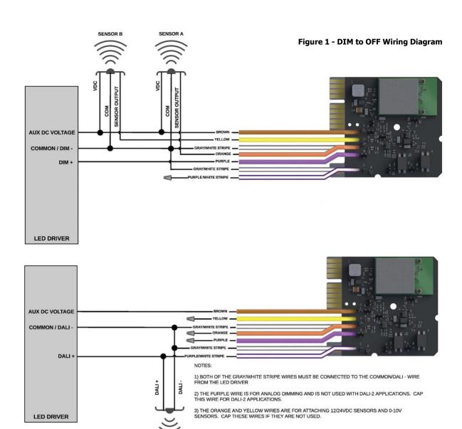
Figure 2 - DALI-2 Wiring Diagram
