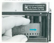
4. While pressing film gently against the sprocket, actuate film advance lever slowly until the perforations on both edges of the film are engaged with sprocket teeth. Then close the back cover.
