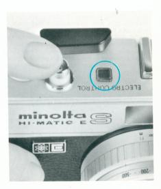
Since lighting of the EE indicator lamp in the viewfinder is also an indication that there is adequate battery power, your Hi-maticES actually gives you battery check information automatically before every exposure.
