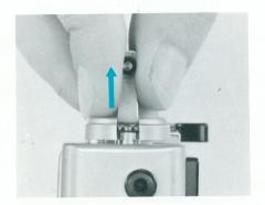
Place film cartridge into the film cartridge chamber. If film rewind key does not engage properly in end of cartridge, rotate film crank in either direction until it does so.
