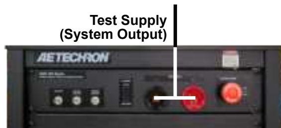
Figure 2.5 – Test Supply Connections (DSR 100 System Output)
