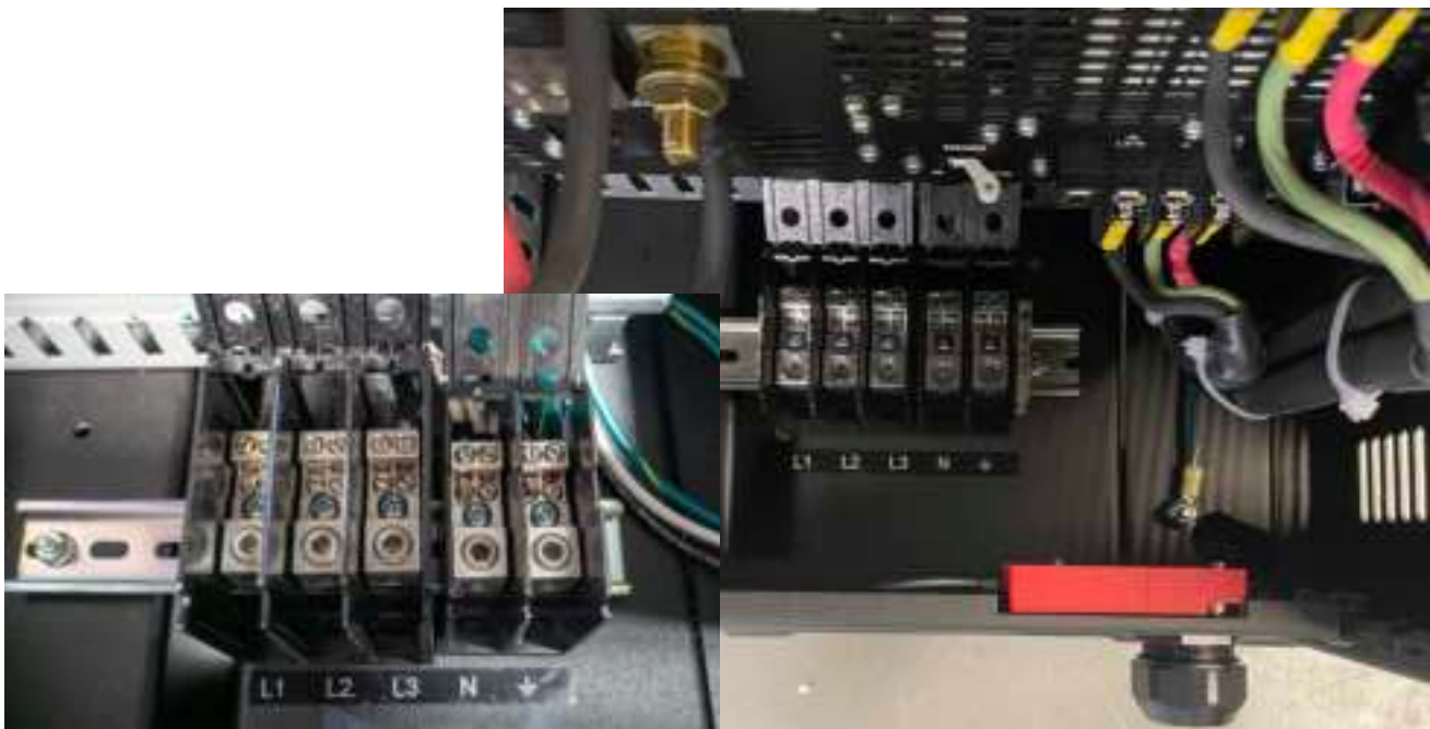
Figure 2.7 – Wiring the AC distribution block
