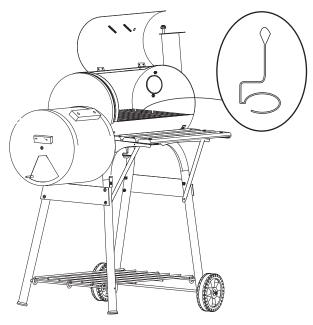
To install the drip tray, feed the base of the holder through the inside of the BBQ base from the inside out.
