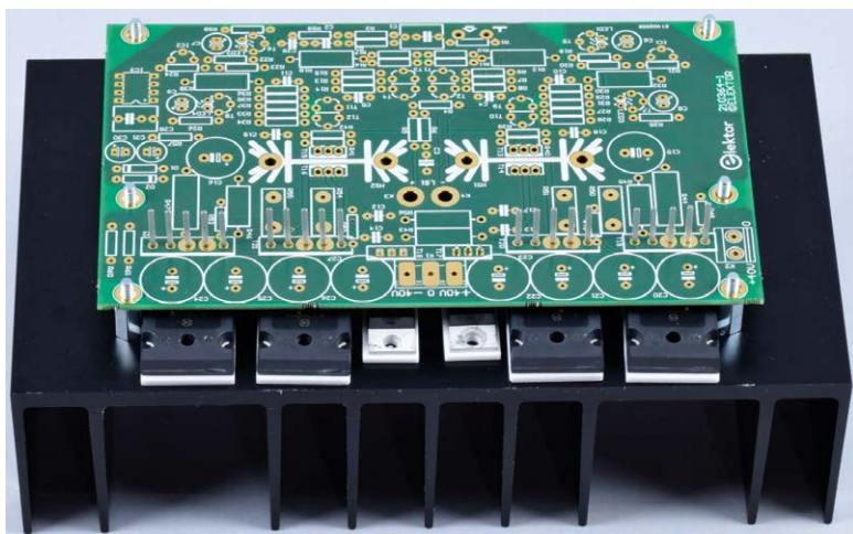
Figure 14. Preparations for marking the 3-mm holes required for the transistors.
