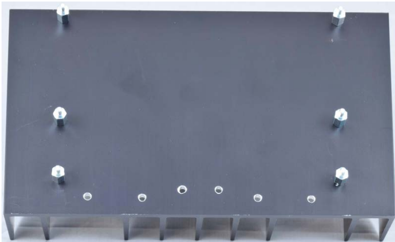
Figure 16. Six 3-mm holes drilled for the transistors in the output stage.
